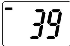
The countdown starts at 50. When the countdown reaches 00 the meter will set its sensor to zero and display CO concentration using three digits. A battery level indicator will appear in the top left hand of the screen and “ppm” will appear in the bottom right hand of the screen
