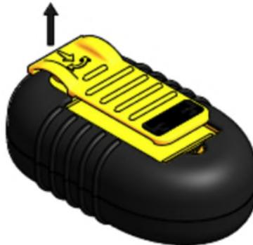
Lift the clip at the pivot end against the spring by a few millimetres and then rotate the clip clear of the battery compartment.
